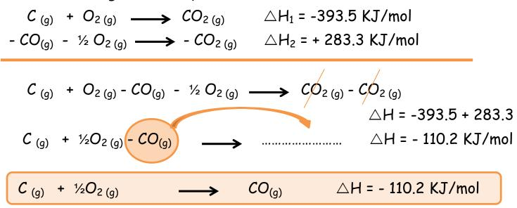
This is the required reaction for formation of carbon monoxide CO
